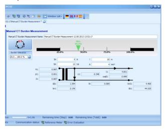
With the **Device Communication** CALegration® allows the user to readout measurement results stored in portable test devices or to preload (Administrative database elements Data. Meters. Instrument Transformers, Test Procedures, Test Point Elements) into the test devices.
